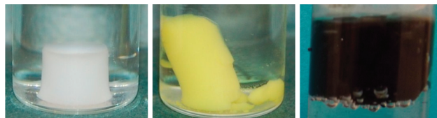
Figure 2. Pictures of a (left) ZnS wet gel and (middle) \text{Cd}^{2+} - and (right) \text{Pb}^{2+} -exchanged wet gels, showing the specific color change and the conservation of the 3D gel monolith integrity upon the cation exchange. (The size of the monoliths is not to scale, nor does it represent a series in which a particular ZnS monolith was exchanged).
